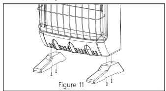
Note: Feet should have long end going out the front of heater, and the edge coinciding with side of heater. If feet overhang side of the heater, switch leg location.
