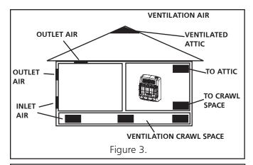
\*IMPORTANT: Do not provide openings for inlet or outlet into attic. If attic has a thermostat-controlled power vent, heated air entering the attic will activate the power vent.
