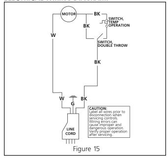
If any original wiring as supplied with the heater must be replaced, it must be replaced with type AWG 105°C wire or its equivalent except as indicated. WARNING: Electrical Grounding Instructions: This heater is equipped with a three-prong (grounding) plug for your protection against shock hazard and should be plugged into a properly grounded three prong receptacle.
